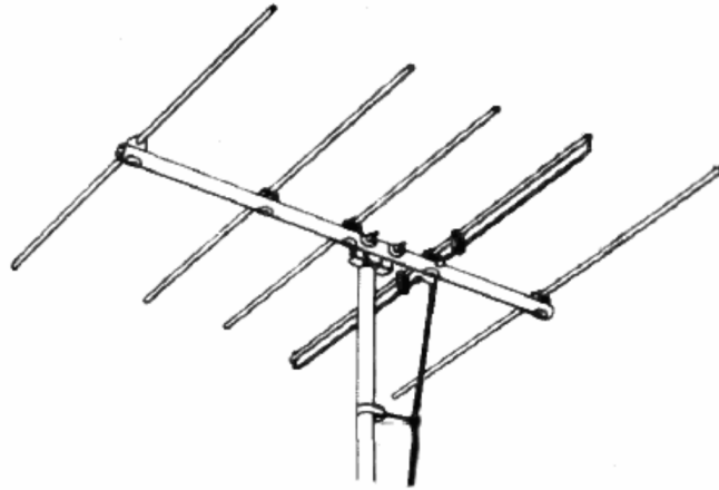
Figure 28.2: In a Yagi-Uda antenna, when a wire antenna is less than half a wavelength, it acts as a waveguide, or a director. Then the wire antenna is slightly more than half a wavelength, it acts as a reflector [130]. Therefore, the antenna radiates predominantly in one direction (courtesy of Wikipedia [131]).
